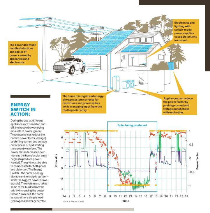
put at lower voltage. Unfortunately, those high frequencies in the power supply can show up as spikes of current in the mains, contributing to harmonic distortion.
